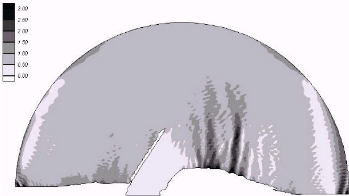
Figure 25. Estimated wave height diagram for normal incident direction, 15-second period wave condition
